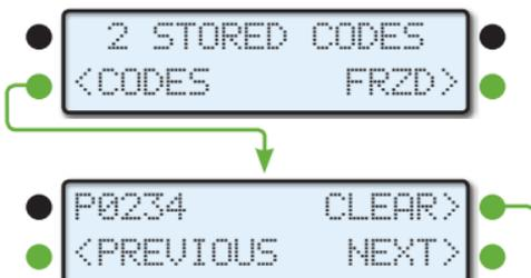
Push the function button next to CLEAR to clear the code and turn off the Check Engine Light.
