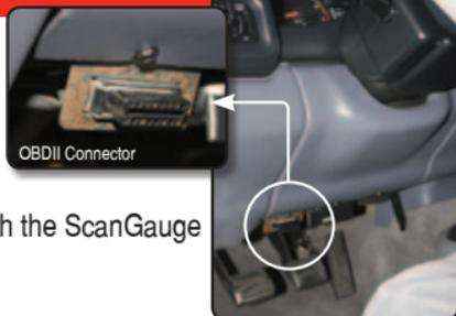
Typical OBDII Connector location
